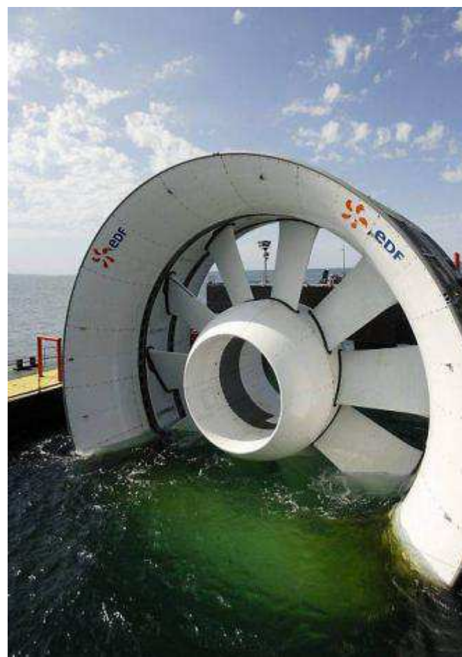
Figure 3: Prototype hydrokinetic turbine tested at Paimpol
